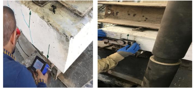
Fig. 4 testing of slabs.
